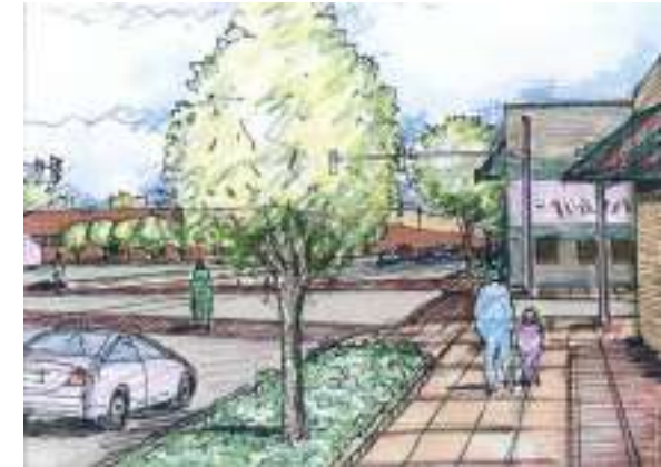
Street trees need at least eight feet of ground exposed to air and water to thrive
