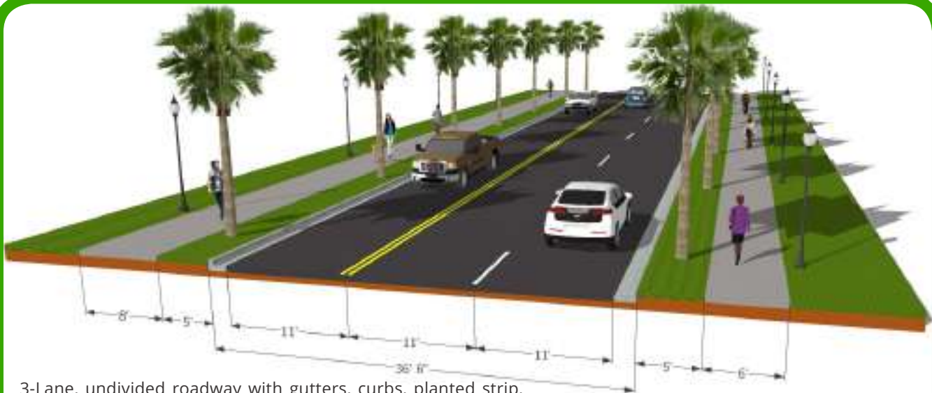
3-Lane, undivided roadway with gutters, curbs, planted strip, and pedestrian level lighting on both sides, and a sidewalk and a multiuse sidepath on opposite sides
