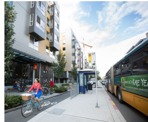
Floating bus stop boarding island (Source: NACTO)
