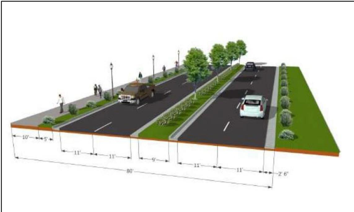
**Figure 2-40: US 52 Cross Section**
