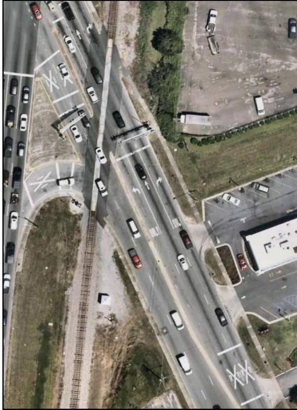
Figure 6 – Red Bank Road Crossing Pavement Markings
