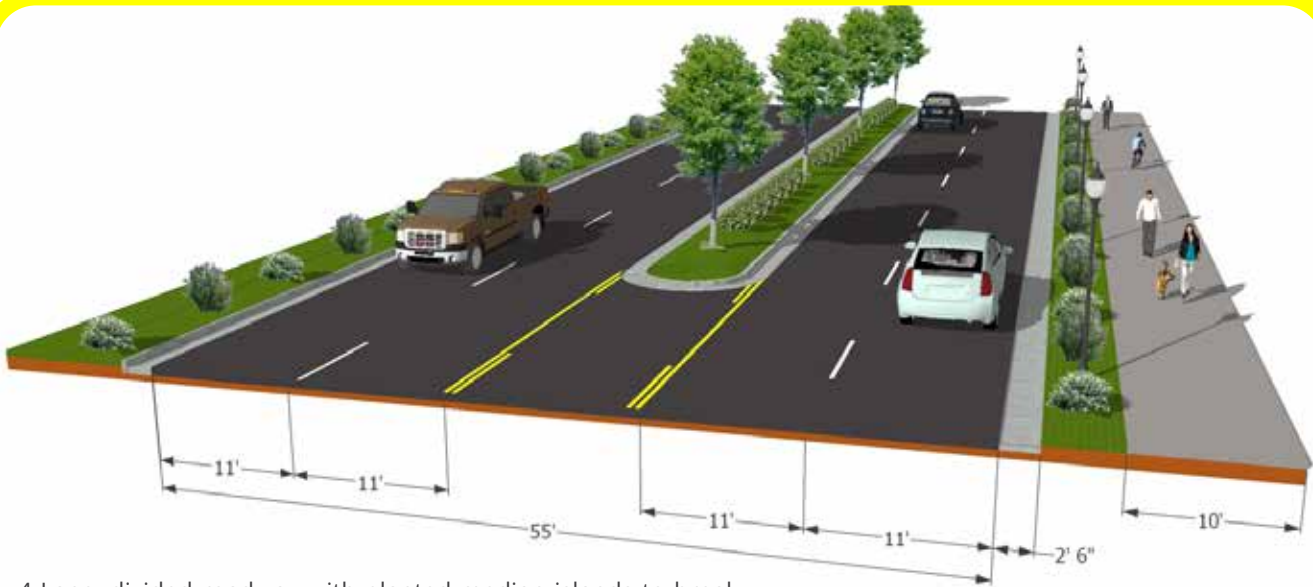
4-Lane, divided roadway with planted median islands to break up turning lane, gutters, curbs, planted strip on both sides and pedestrian level lighting and sidewalk on one side
