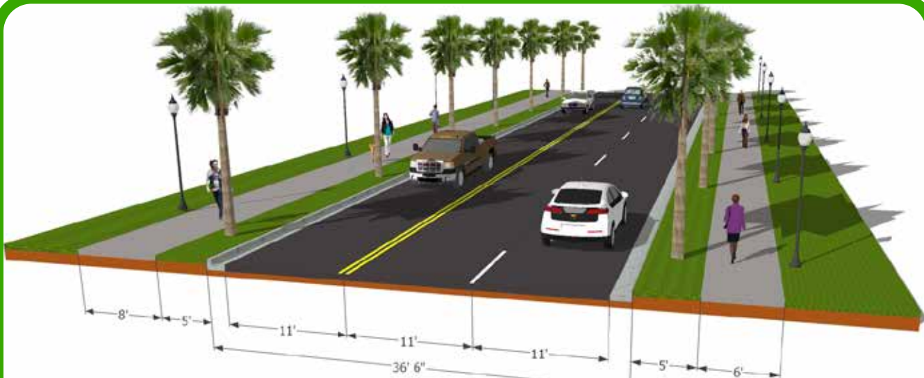
3-Lane, undivided roadway with gutters, curbs, planted strip, and pedestrian level lighting on both sides, and a sidewalk and a multiuse sidepath on opposite sides
