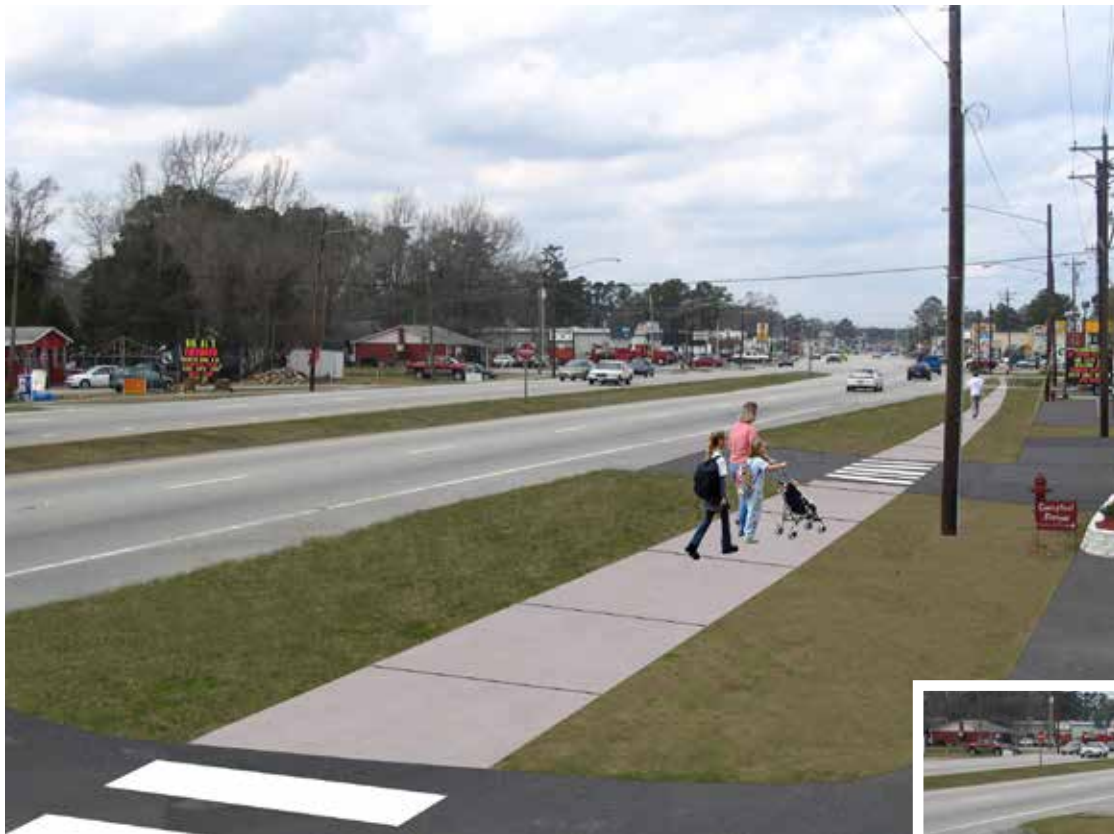
An example of how an existing street (below) could be redesigned with access management, driveway consolidation, and pedestrian infrastructure (left).
