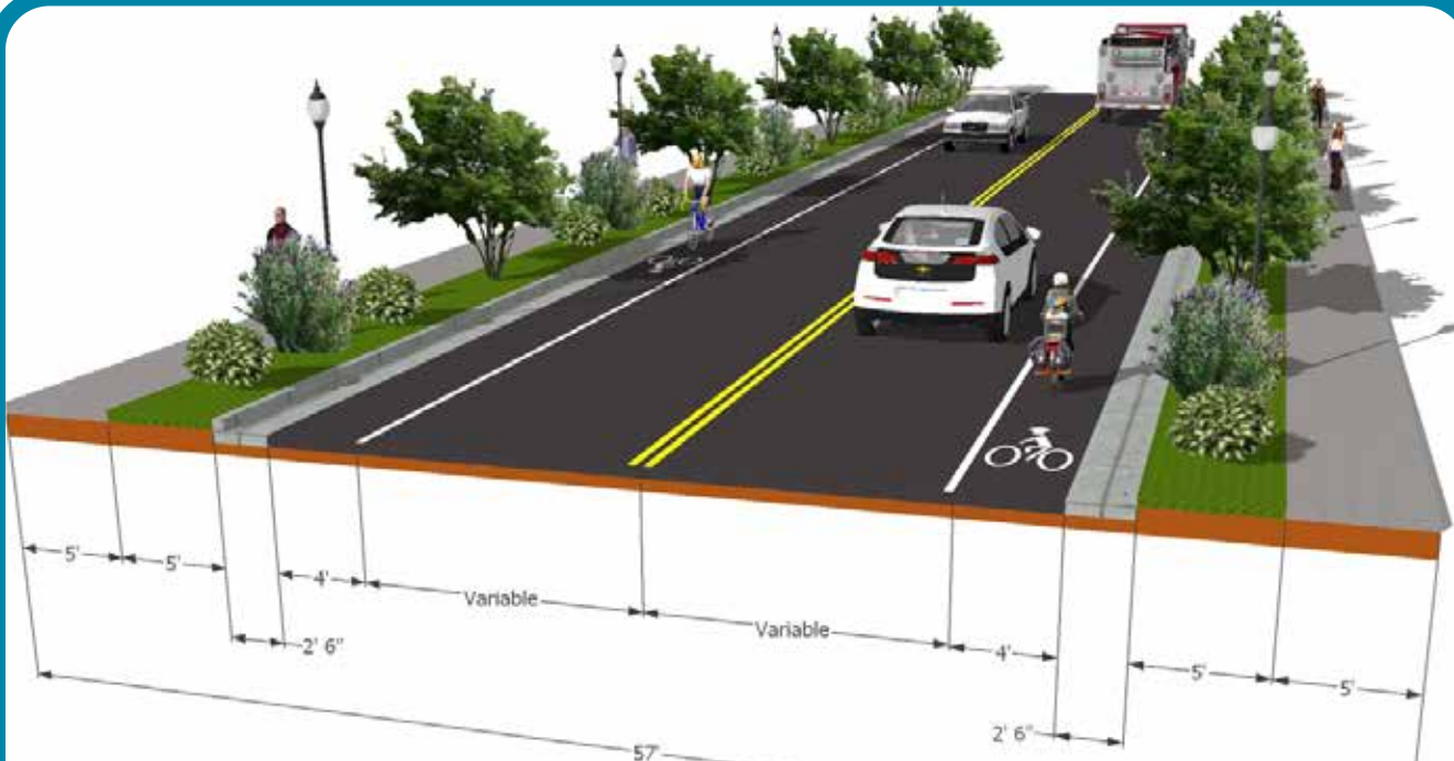
2-Lane, undivided roadway with bicycle lanes, curbs, gutters, and sidewalks on both sides
