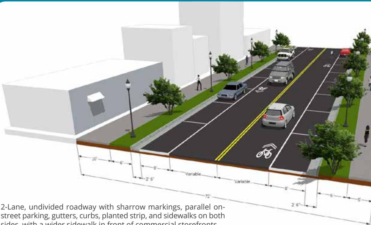
2-Lane, undivided roadway with sharrow markings, parallel on-street parking, gutters, curbs, planted strip, and sidewalks on both sides, with a wider sidewalk in front of commercial storefronts
