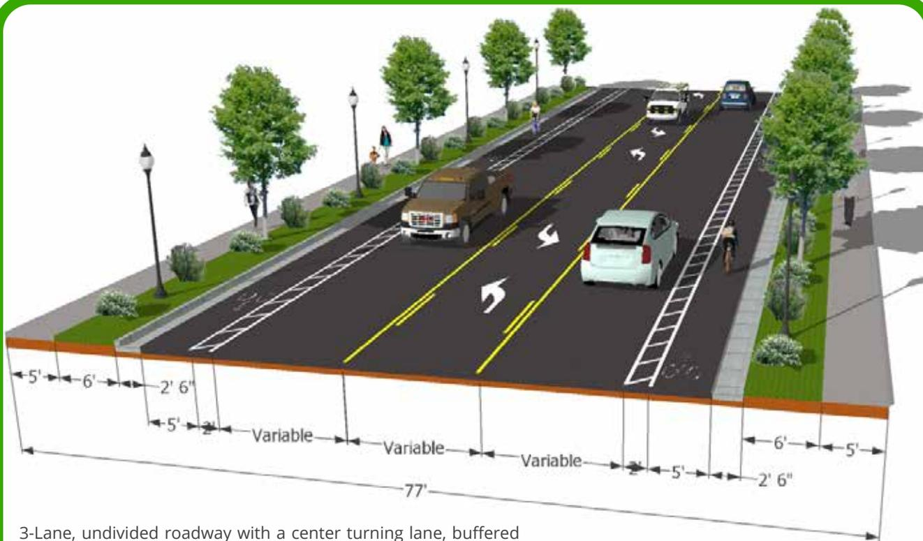
3-Lane, undivided roadway with a center turning lane, buffered bicycle lanes, curbs, gutters, planted strips, , pedestrian level lighting and sidewalks on both sides
