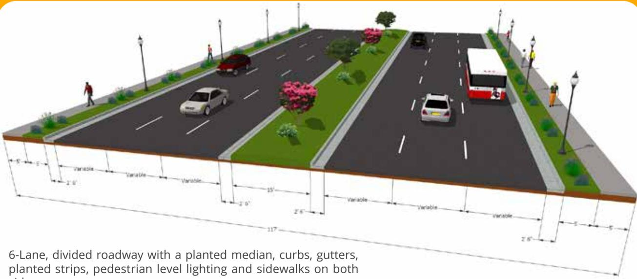
6-Lane, divided roadway with a planted median, curbs, gutters, planted strips, pedestrian level lighting and sidewalks on both sides
