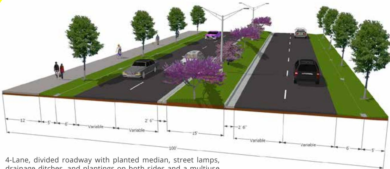
4-Lane, divided roadway with planted median, street lamps, drainage ditches, and plantings on both sides and a multiuse sidepath on one side.
