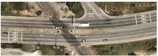
Figure 29 - Ashley Phosphate Crossing Pavement Markings
