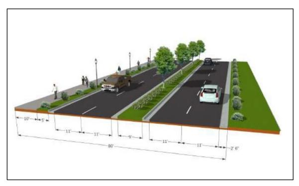
Figure 2-40: US 52 Cross Section
