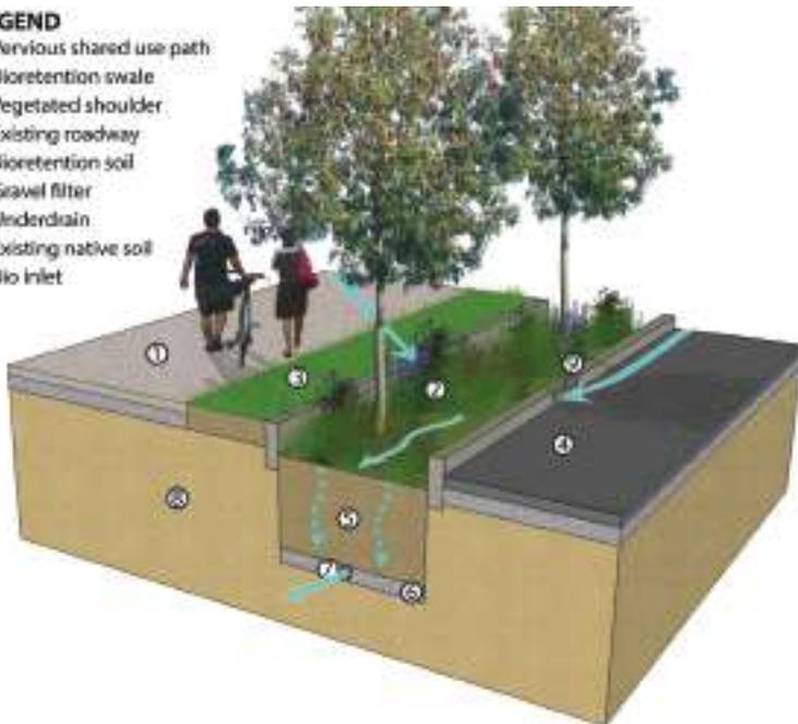
above: Town bioretention “typical” – encourages infiltration in areas of well draining soils
