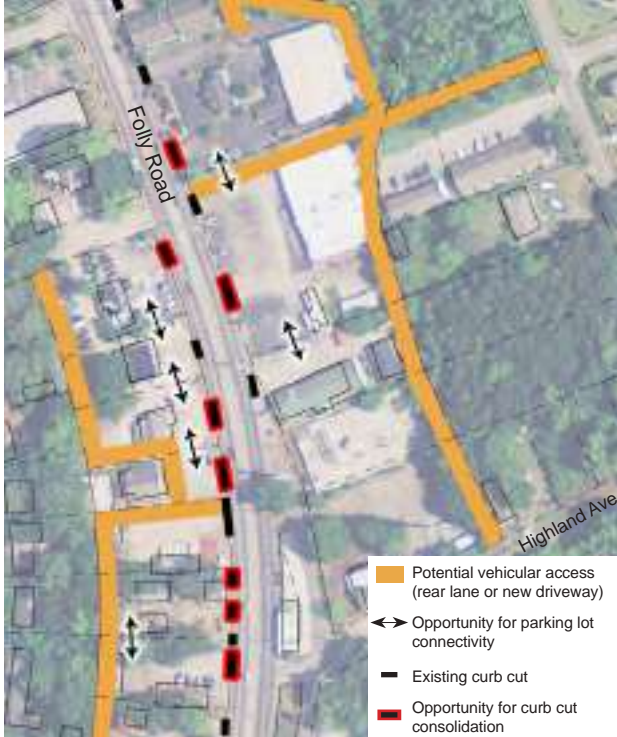
above: Preliminary analysis of potential curb consolidation and cross-access opportunities in the Commercial Core area
