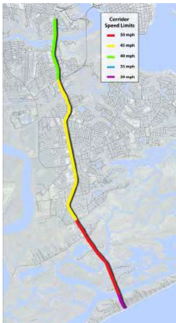
below: Existing speed limits. Note: A speed study on a portion of Folly Road was conducted in the summer of 2015, which resulted in the reduction of the 50 mph section to become 45 mph.
